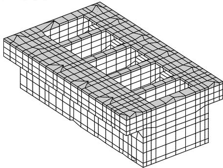
Figure 1: 7980 DOF engine block model used for the detailed accuracy evaluation.
