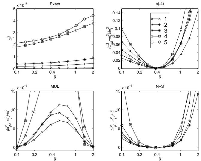
Figure 2: Evolution of *frequencies* and relative error on frequencies predicted by reduced models (16 modes computed for  $\beta = .4$ , MUL, and N+S)
