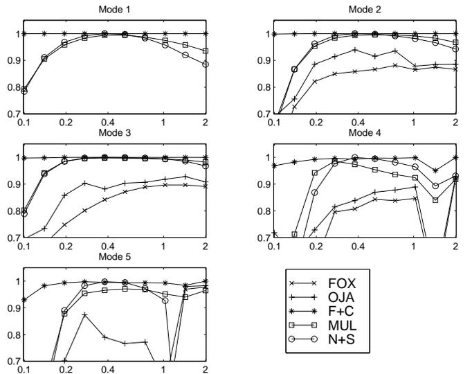
Figure 6: Evolution of  $MAC_M(\partial\phi_{jR}/\partial p, \partial\phi_j/\partial p)$  for the first 5 flexible modes and the different methods
