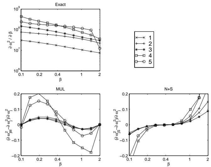
Figure 3: Evolution of *frequency sensitivities* and relative error on frequency sensitivities predicted by reduced models
