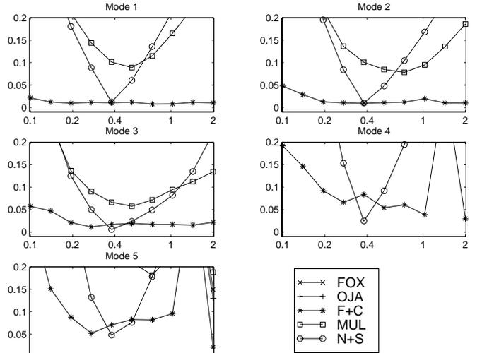
Figure 5: Evolution of  $rel_K(\partial\phi_{jR}/\partial p, \partial\phi_j/\partial p)$  for the first 5 flexible modes and the different methods
