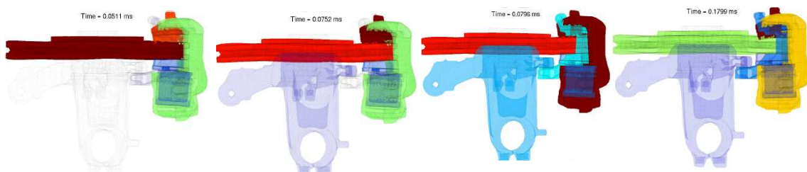
Figure 11: Evolution of the component strain energy repartition as function of time in the limit cycle.
