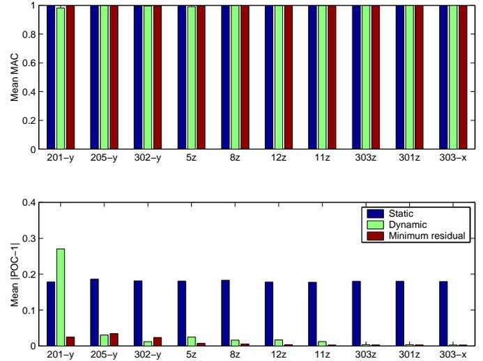
**Figure 6: Impact of neglecting sensor/FEM node distance on various sensors when using static, dynamic and minimum residual expansion.**
