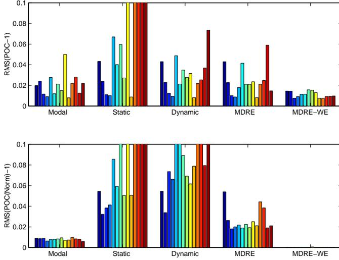
**Figure 8: Impact on expansion results of random noise added to modeshapes**
