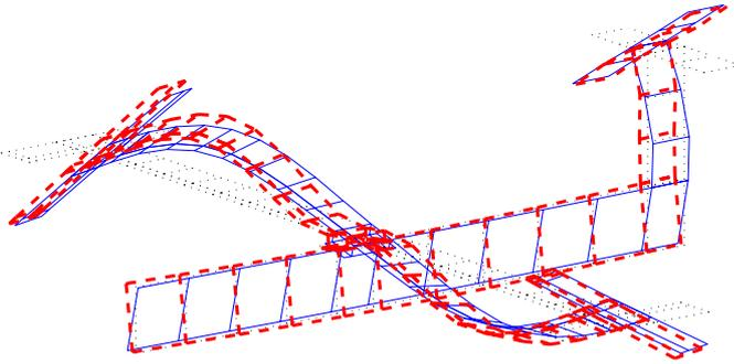
**Figure 5: Problem with modal expansion : the strong bending near the wing/fuselage connection is not physical**
