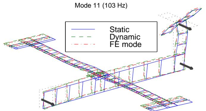
**Figure 7: Problems with static : the two horizontal sensors cannot capture fuselage bending for static expansion.**
