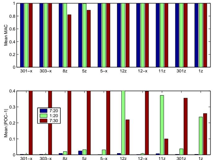
Figure 4: Impact of neglecting sensor/FEM node distance on various sensors when using modal expansion and different target mode selections
