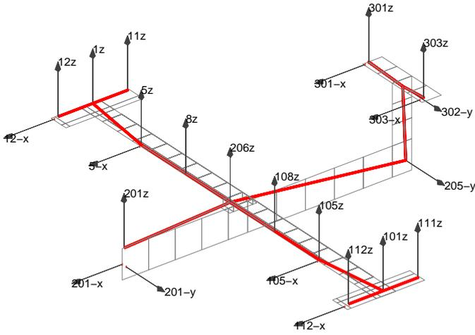
Figure 2: Sensor configuration, wire-frame display and FEM mesh.
